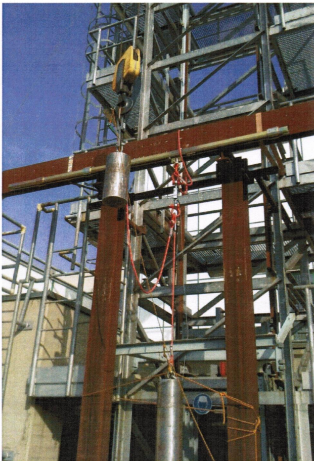
m_{\text{dyn}} = 100 \text{ kg} , m_{\text{stat}} = 200 \text{ kg} , h_{\text{fall}} = 2,65 \text{ m}
